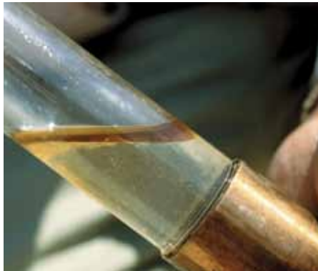
Above Transparent borehole sampling tube (bailer) showing layer of fuel oil contamination floating on top of groundwater. Kwinana, WA.
