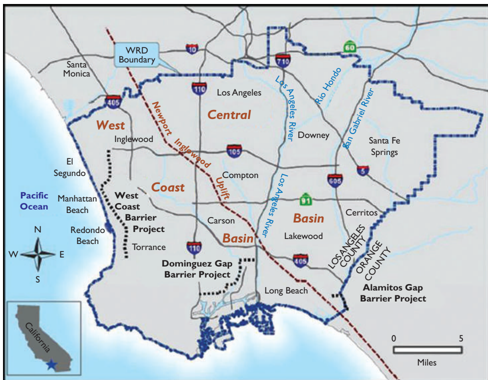
Figure 7.7 The three seawater intrusion barriers to protect groundwater in the Los Angeles coastal area, California, USA. [Source: Johnson (2007)].
