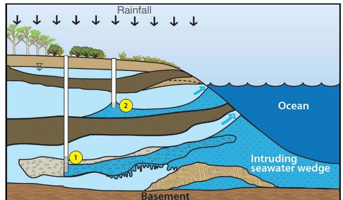
The image above shows seawater intrusion occurring in a more complex aquifer with human activity contributing. The image shows (1) seawater moving preferentially through high-permeability layers in the ground, and (2) excessive pumping drawing seawater upwards, causing the bore to become contaminated.
