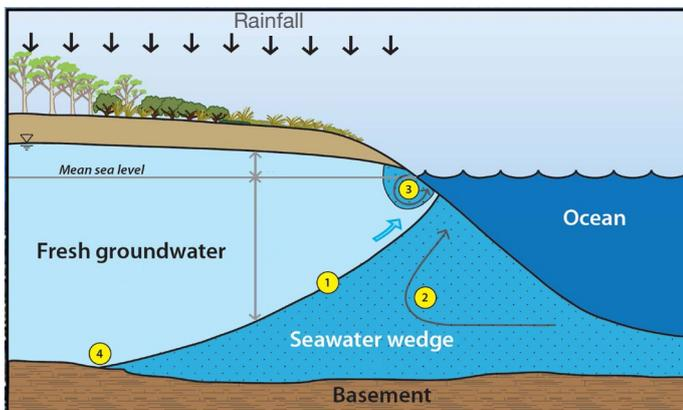
The image above shows the natural equilibrium of seawater and groundwater in an undisturbed system. Figure (1) marks the interface between seawater and groundwater; (2) shows movement of water affected by density, while (3) is movement driven by the tide. Figure (4) shows the furthest extent of seawater intrusion.
